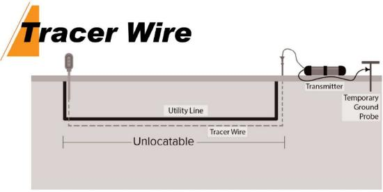
Tracer wire not properly grounded results in a missing signal and incomplete circuit.
