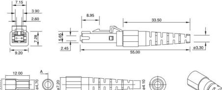
QS type, quick assembly SC connector kits, for 3.0mm round cable
